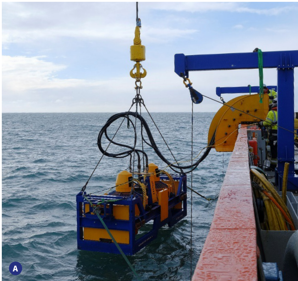
A Deployment of Controlled Flow excavation tool
