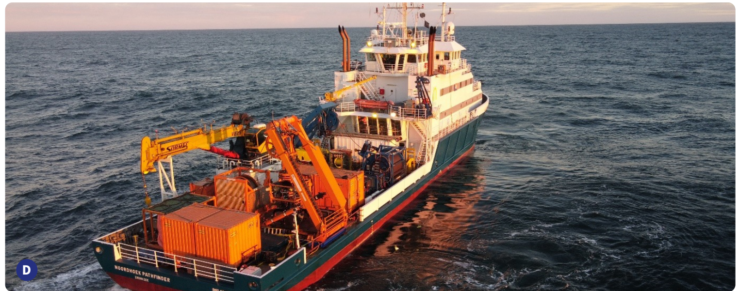
A Deployment of ROV Grab B LARS including grab system C Boulder located on the seabed D Pathfinder with UTROV installed on the aft
