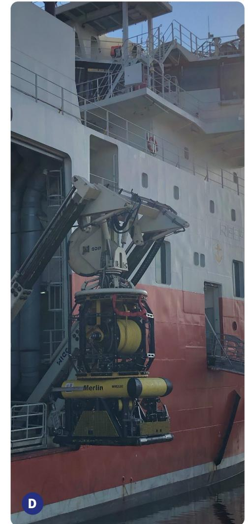
**A** An N-Sea owned dive spread installed on board OSV Larissa **B** Replaced cable protection system elements **C** OSV Larissa **D** Over boarding of WROV
